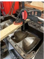
a clamp down in the hole where the oil pump goes in and the other end of the clamp on top of the board. The tray pops right out. There are sharp edges on the tray with the baffles on the underside, be careful. Before you snap the tray back in make sure all of the old gasket material is cleaned from the surface and the lip of the tray fits properly on both sides.
